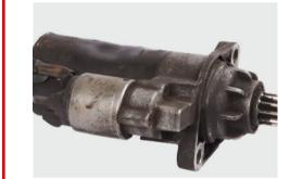
Severely deformed housing
