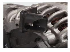
Plug damaged below sealing ring
